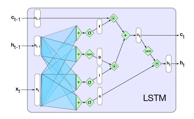
A single LSTM unit displayed as a computation graph. The inputs to each unit consists of the current input, x, the previous hidden state  $h_{t-1}$ , and the previous context  $c_{t-1}$ , . The outputs are a new hidden state,  $h_t$  and an updated context,  $c_t$ .
