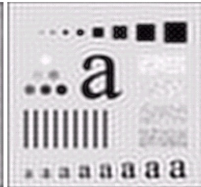
Result of filtering with ideal low pass filter of radius 30
