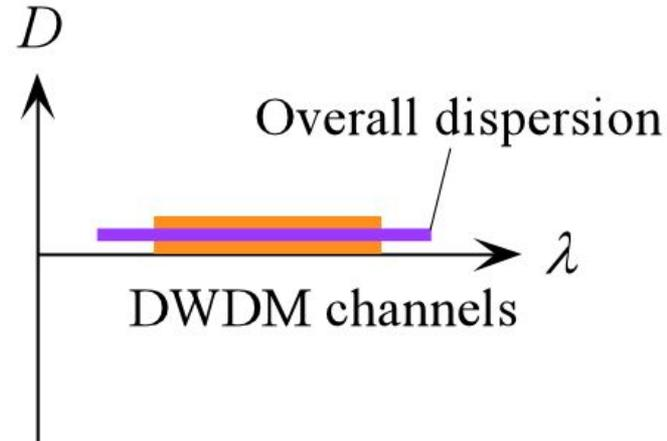
Dispersion  $D$  vs. wavelength characteristics involved in dispersion compensation. Inverse dispersion fiber enables the dispersion to be reduced and maintained flat over the communication wavelengths.
