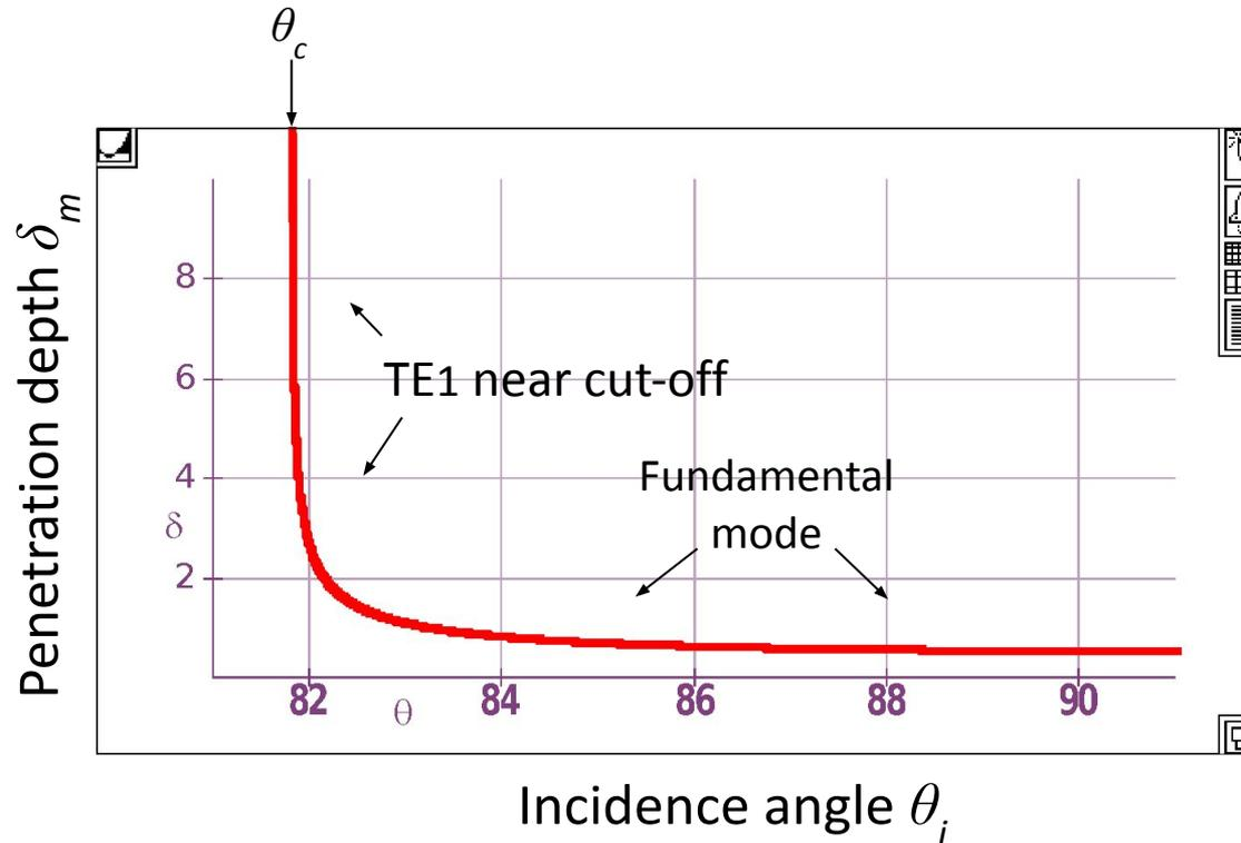
The mode  $TE_1$  penetrates into the cladding where its velocity is higher than in the core. If penetration is large, as near cut-off,  $TE_1$  group velocity along the guide can exceed that of  $TE_0$ .
