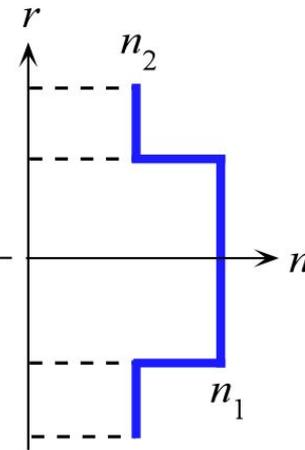
(a) Multimode step index fiber. Ray paths are different so that rays arrive at different times.
