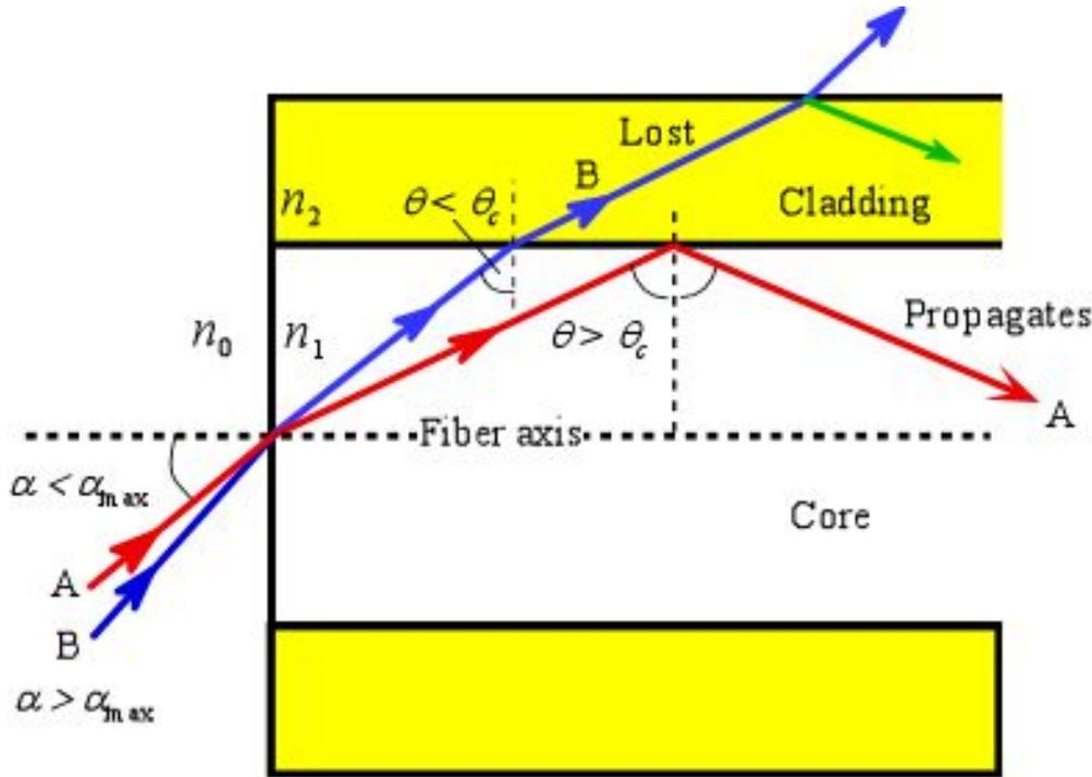
Maximum acceptance angle  $\alpha_{max}$  is that which just gives total internal reflection at the core-cladding interface, i.e. when  $\alpha = \alpha_{max}$  then  $\theta = \theta_c$ . Rays with  $\alpha > \alpha_{max}$  (e.g. ray B) become refracted and penetrate the cladding and are eventually lost.
