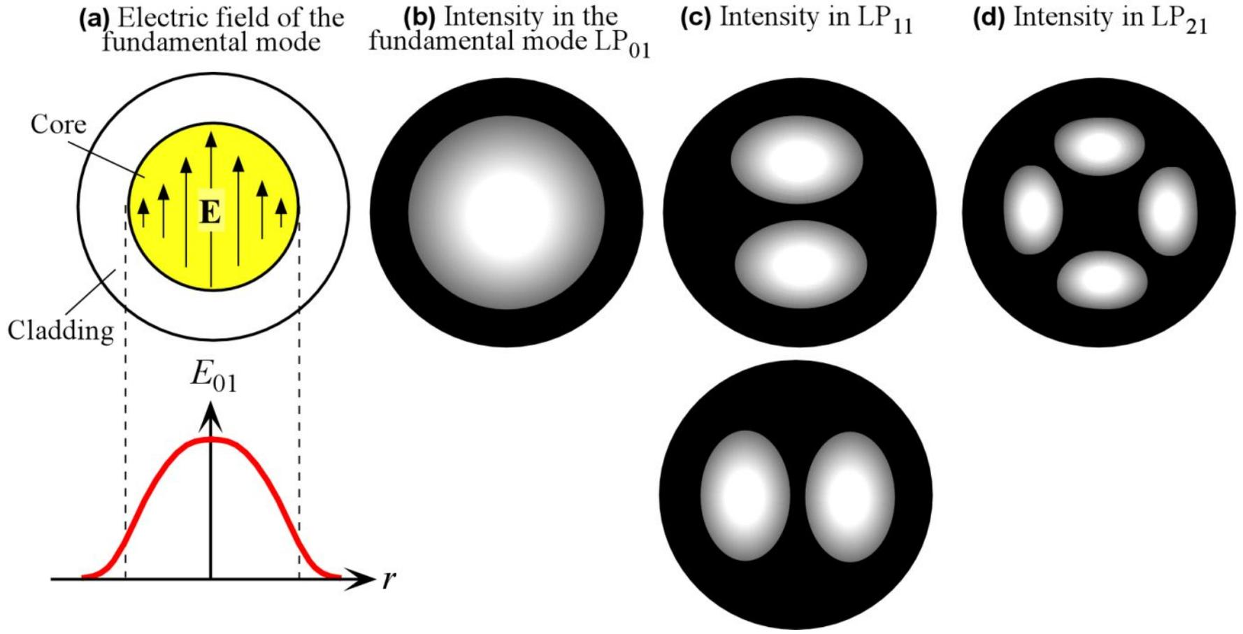
The electric field distribution of the fundamental mode in the transverse plane to the fiber axis  $z$ . The light intensity is greatest at the center of the fiber. Intensity patterns in  $LP_{01}$ ,  $LP_{11}$  and  $LP_{21}$  modes. (a) The field in the fundamental mode. (b)-(d) Indicative light intensity distributions in three modes,  $LP_{01}$ ,  $LP_{11}$  and  $LP_{21}$ .
