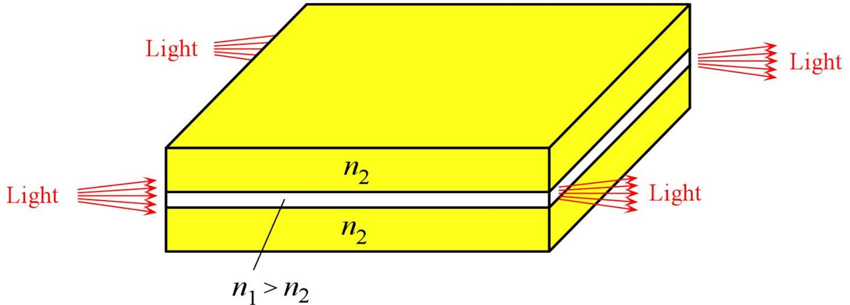
A planar dielectric waveguide has a central rectangular region of higher refractive index  $n_1$  than the surrounding region which has a refractive index  $n_2$ . It is assumed that the waveguide is infinitely wide and the central region is of thickness  $2a$ . It is illuminated at one end by a nearly monochromatic light source.
