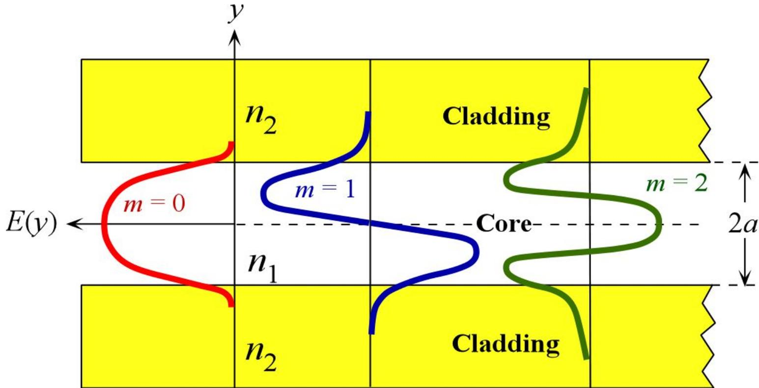
The electric field patterns of the first three modes ( $m = 0, 1, 2$ ) traveling wave along the guide. Notice different extents of field penetration into the cladding
