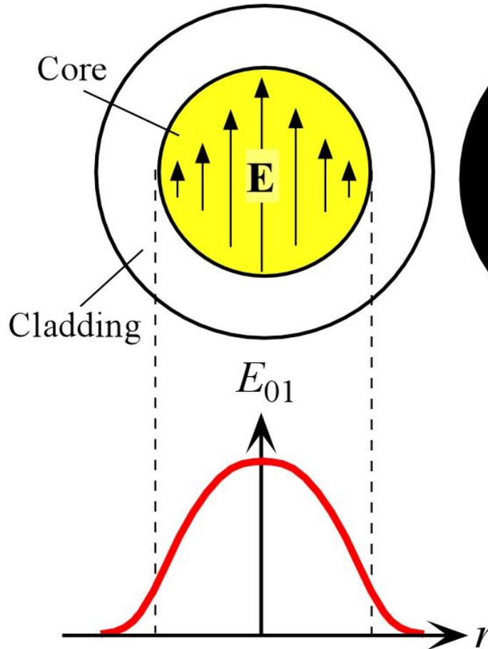
The electric field distribution of the fundamental mode,  $LP_{01}$ , in the transverse plane to the fiber axis  $z$ . The light intensity is greatest at the center of the fiber
