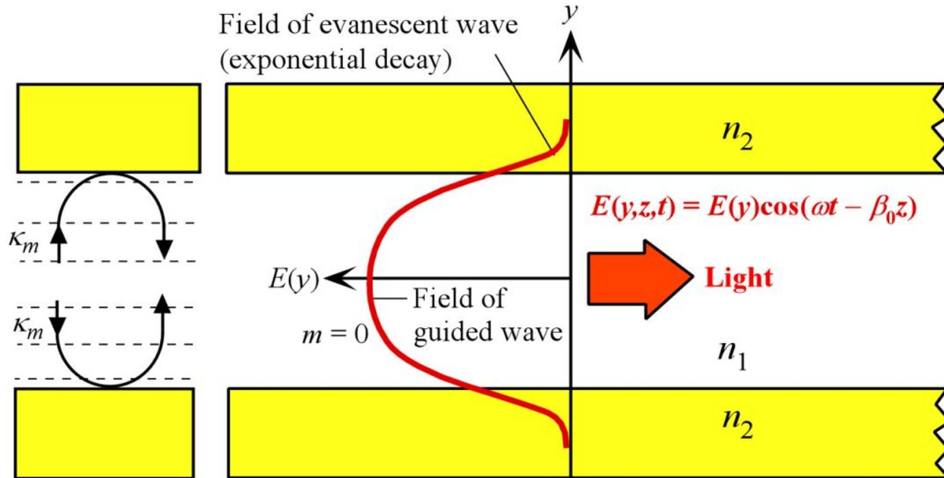
Left: The upward and downward traveling waves have equal but opposite wave vectors  $\kappa_m$  and interfere to set up a standing electric field pattern across the guide.
