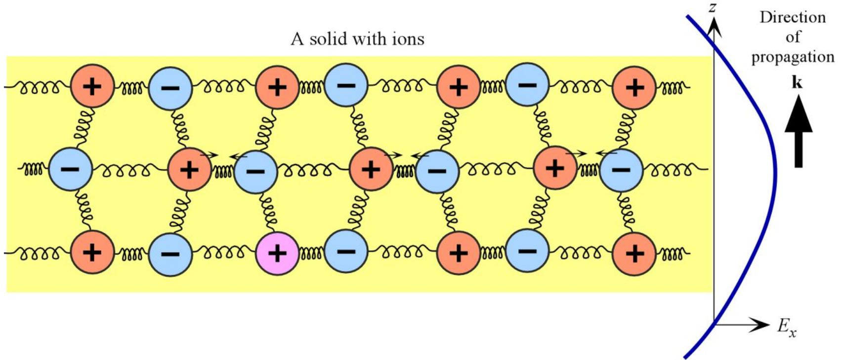
EM Wave oscillations are coupled to lattice vibrations (phonons), vibrations of the ions in the lattice. Energy is transferred from the EM wave to these lattice vibrations.
