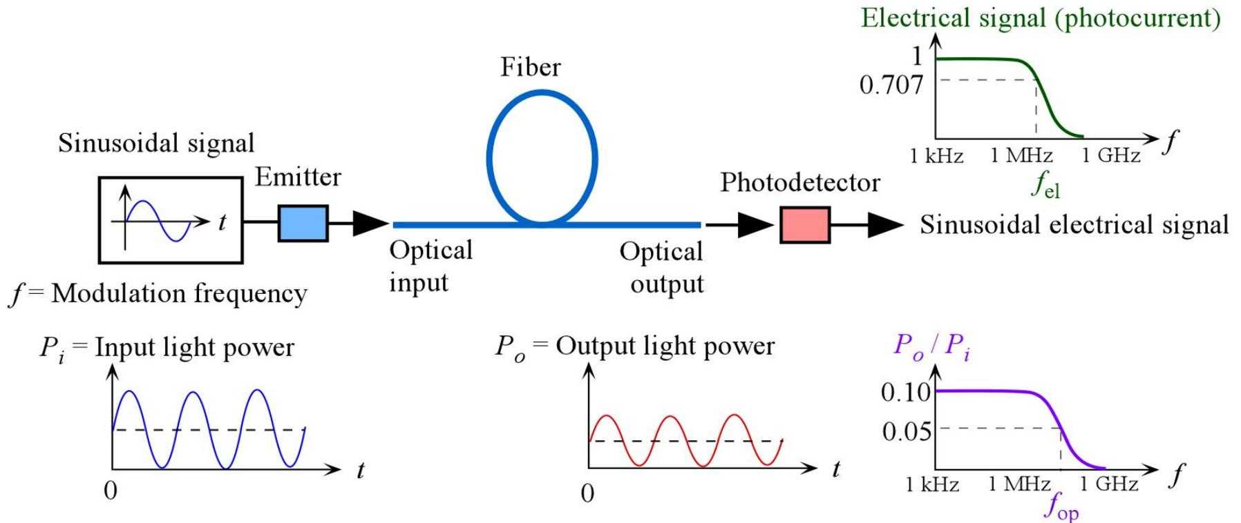
An optical fiber link for transmitting analog signals and the effect of dispersion in the fiber on the bandwidth,  $f_{op}$ .
