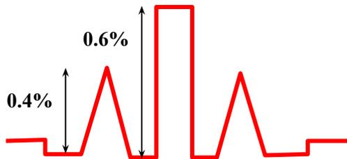
**Fiber with flattened dispersion slope (schematic)**
