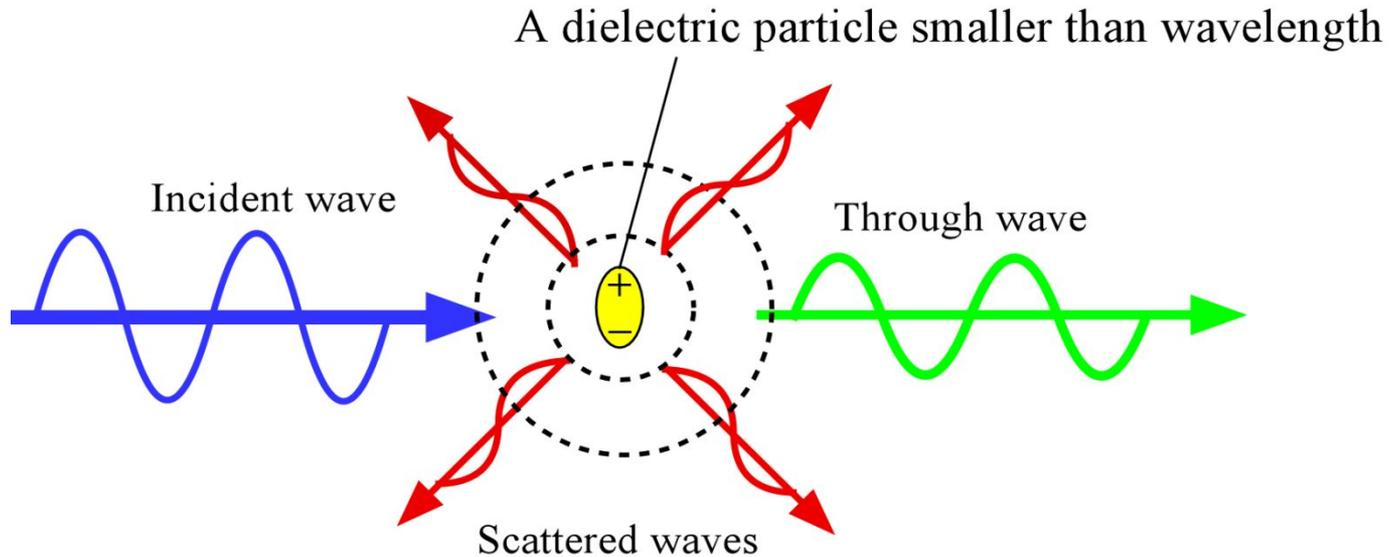
Rayleigh scattering involves the polarization of a small dielectric particle or a region that is much smaller than the light wavelength. The field forces dipole oscillations in the particle (by polarizing it) which leads to the emission of EM waves in "many" directions so that a portion of the light energy is directed away from the incident beam.
