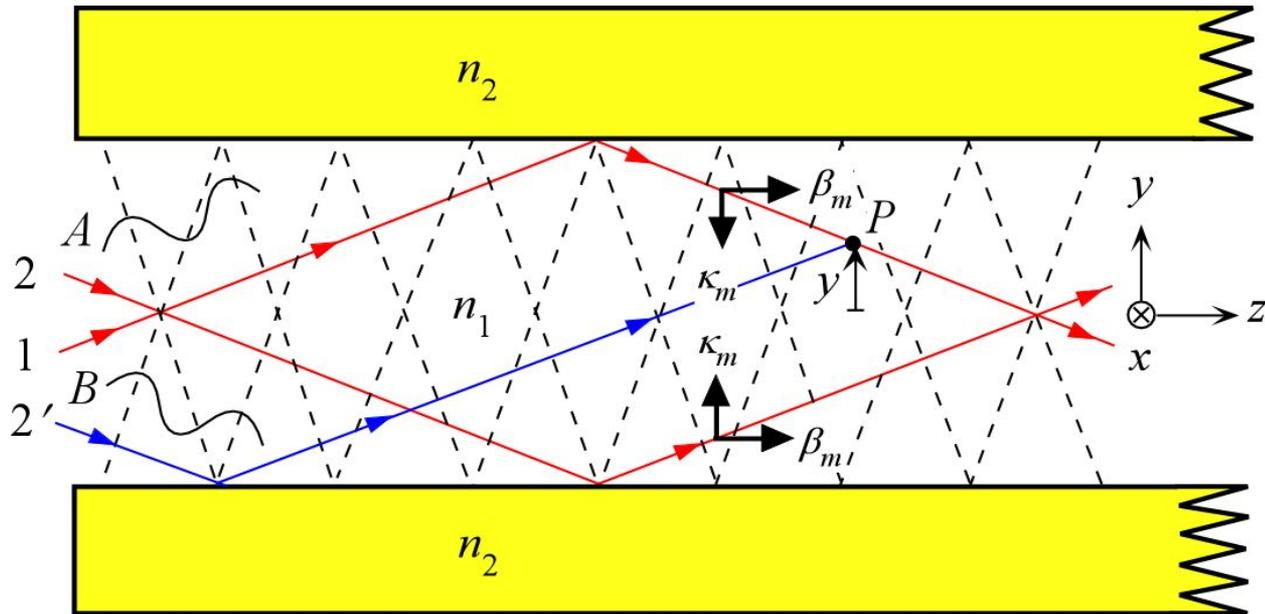
To get a propagating wave along a guide you must have constructive interference. All these rays interfere with each other. Only certain angles are allowed. Each allowed angle represents a **mode** of propagation.
