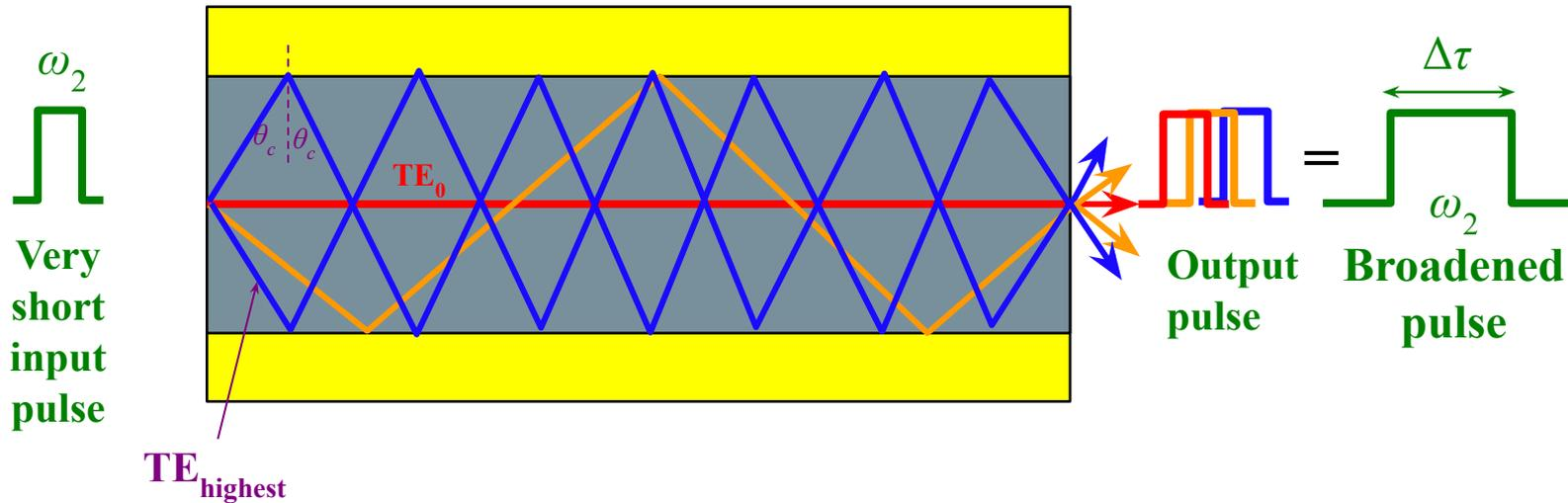
$$\frac{\Delta\tau}{L} = \frac{1}{v_{g\min}} - \frac{1}{v_{g\max}}$$
