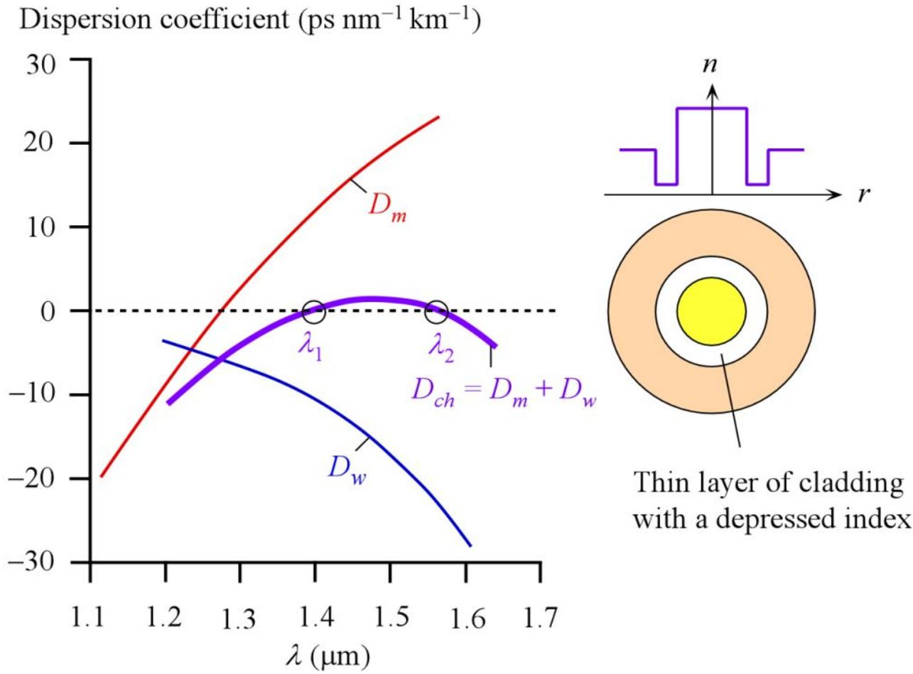
Dispersion flattened fiber example. The material dispersion coefficient ( $D_m$ ) for the core material and waveguide dispersion coefficient ( $D_w$ ) for the doubly clad fiber result in a flattened small chromatic dispersion between  $\lambda_1$  and  $\lambda_2$ .
