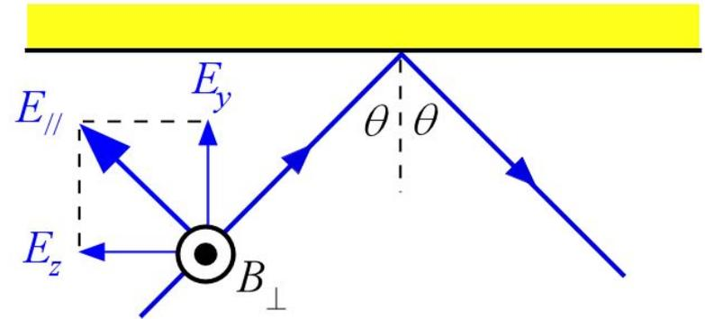
$B_{\perp}$  is along  $-x$ , so that  $B_{\perp} = -B_x$
