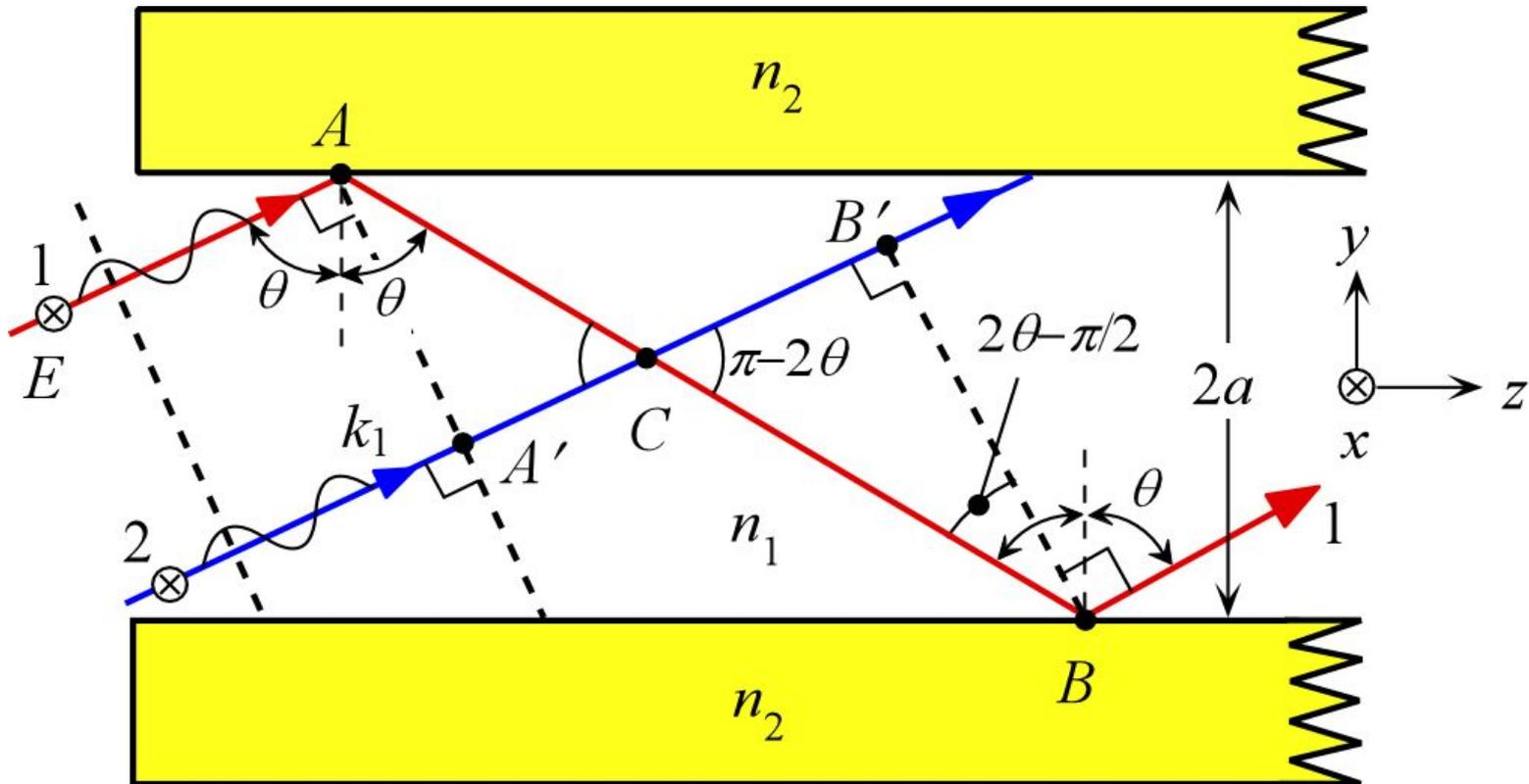
Two arbitrary waves 1 and 2 that are initially in phase must remain in phase after reflections. Otherwise the two will interfere destructively and cancel each other.
