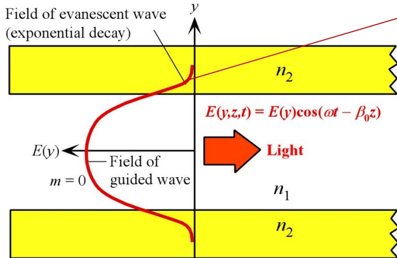
$$E_{\text{cladding}}(y') = E_{\text{cladding}}(0)\exp(-\alpha_{\text{cladding}}y')$$
