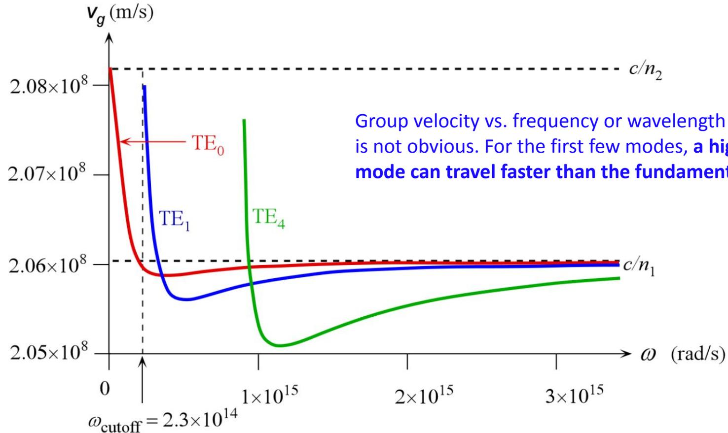
The group velocity  $v_g$  vs.  $\omega$  for a planar dielectric guide with a core thickness ( $2a$ ) =  $20 \mu\text{m}$ ,  $n_1 = 1.455$ ,  $n_2 = 1.440$ .  $\text{TE}_0$ ,  $\text{TE}_1$  and  $\text{TE}_4$
