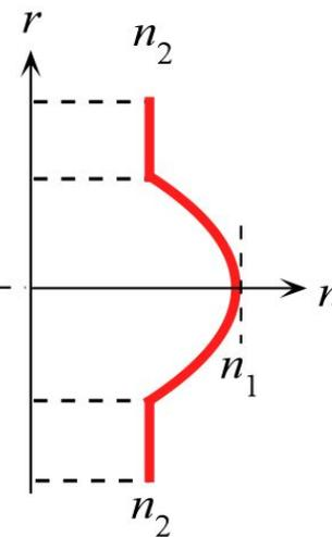
(b) Graded index fiber. Ray paths are different but so are the velocities along the paths so that all the rays arrive at the same time.
