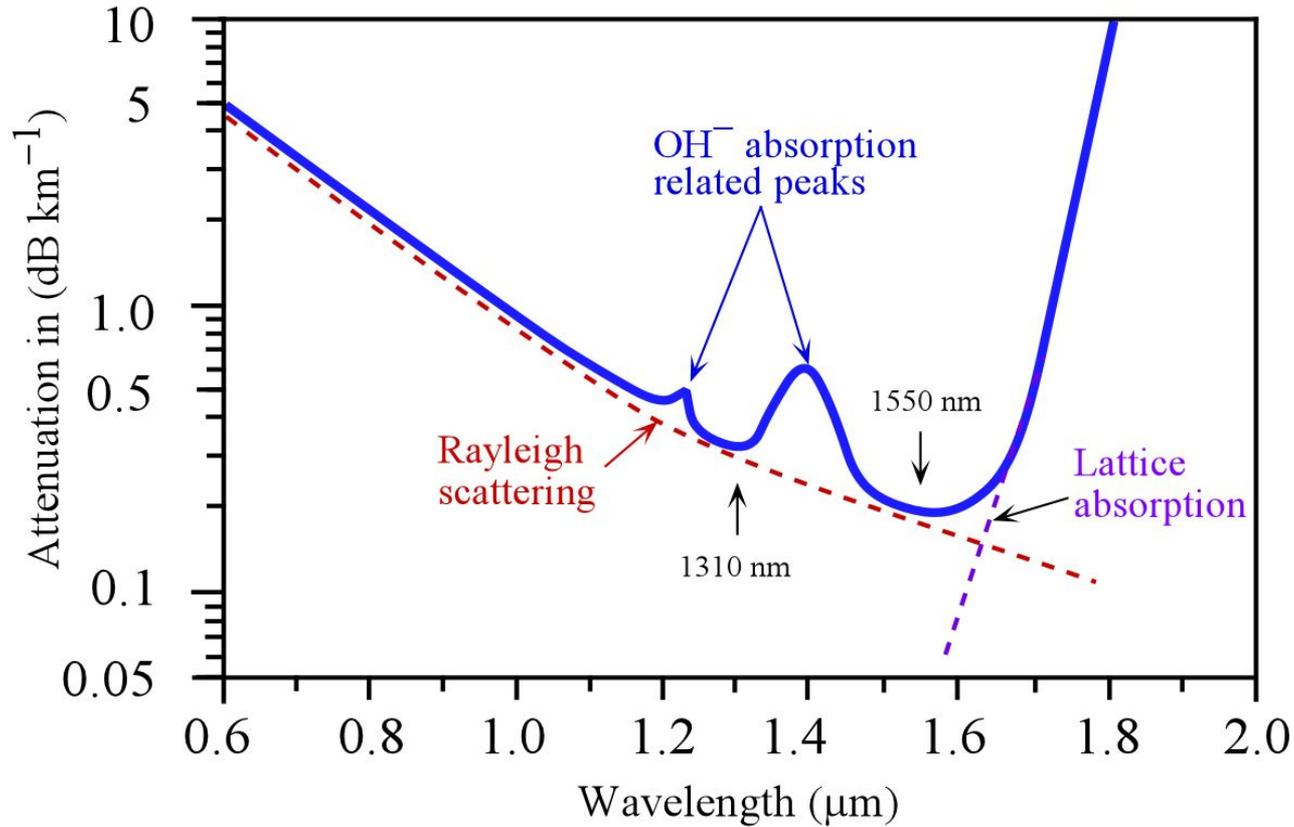
Attenuation vs. wavelength for a standard silica based fiber.
