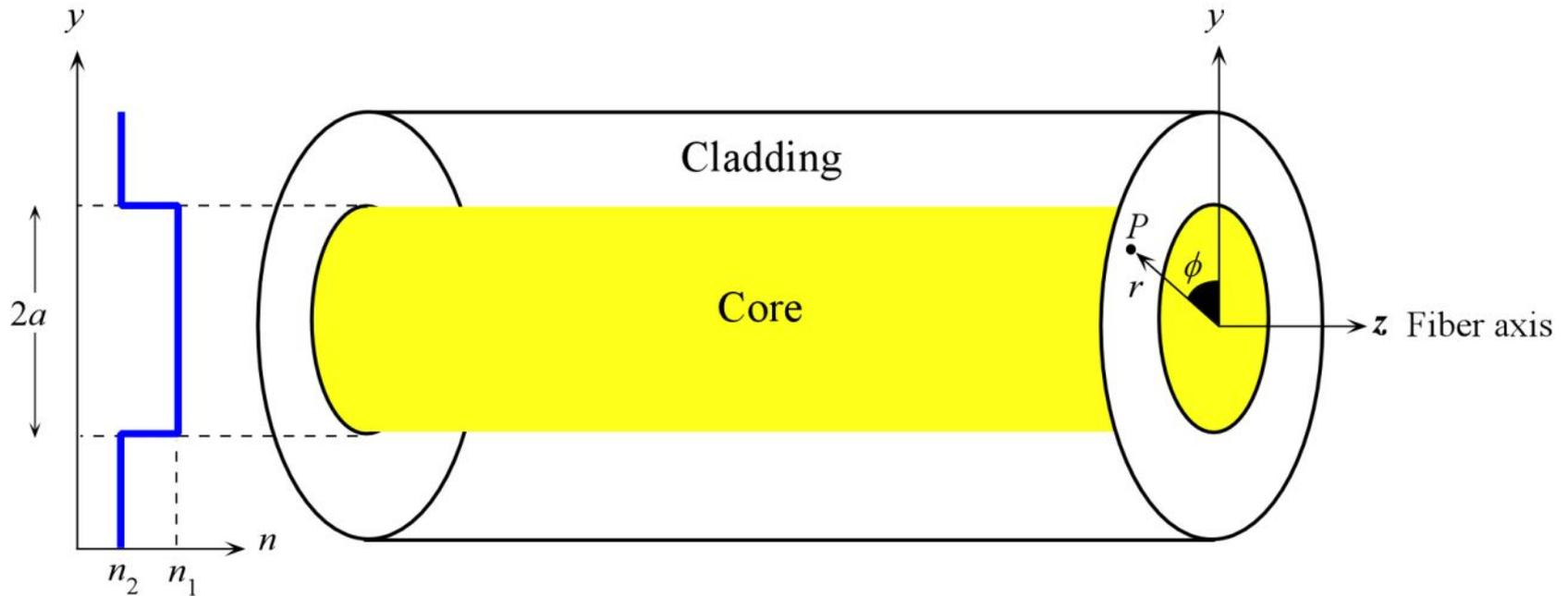
The step index optical fiber. The central region, the core, has greater refractive index than the outer region, the cladding. The fiber has cylindrical symmetry. The coordinates  $r, \phi, z$  are used to represent any point  $P$  in the fiber. Cladding is normally much thicker than shown.
