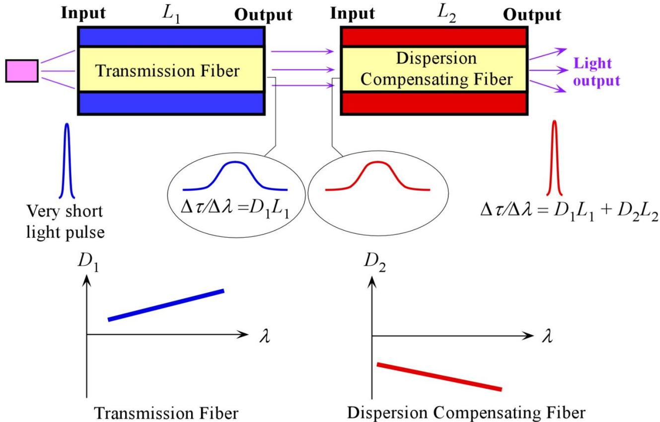
$$\begin{aligned} \text{Total dispersion} &= D_t L_t + D_c L_c = (10 \text{ ps nm}^{-1} \text{ km}^{-1})(1000 \text{ km}) + \\ &\quad (-100 \text{ ps nm}^{-1} \text{ km}^{-1})(80 \text{ km}) \\ &= 2000 \text{ ps/nm for 1080 km} \end{aligned}$$
