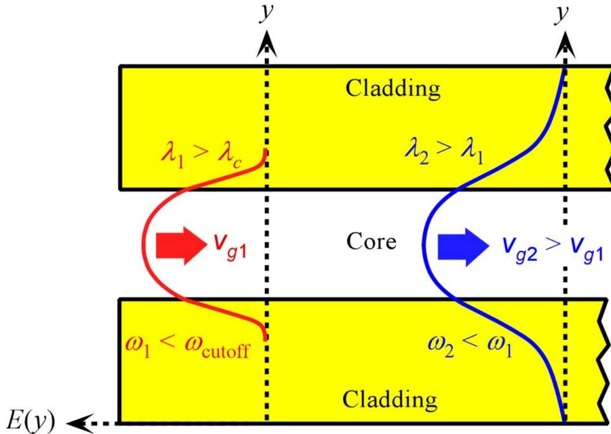
The electric field of TE<sub>0</sub> mode extends more into the cladding as the wavelength increases. As more of the field is carried by the cladding, the group velocity increases.
