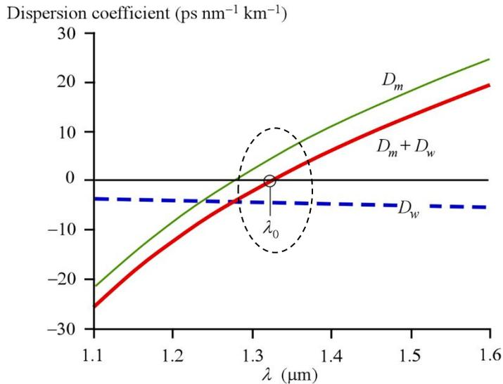
The cause of  $\Delta\tau$  is the wavelength spread  $\Delta\lambda$  at the input
