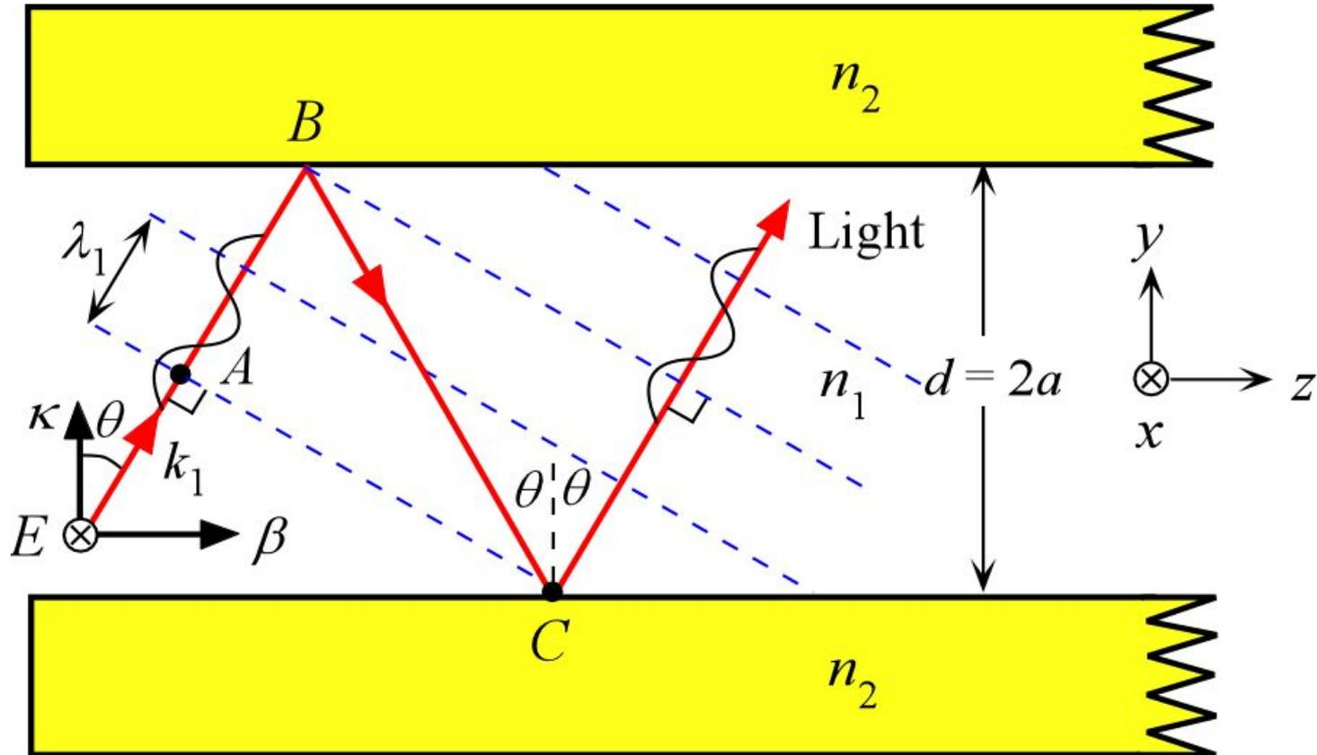
A light ray traveling in the guide must interfere constructively with itself to propagate successfully. Otherwise destructive interference will destroy the wave.  $E$  is parallel to  $x$ . ( $\lambda_1$  and  $k_1$  are the wavelength and the propagation constant inside the core medium  $n_1$  i.e.  $\lambda_1 = \lambda/n_1$ .)
