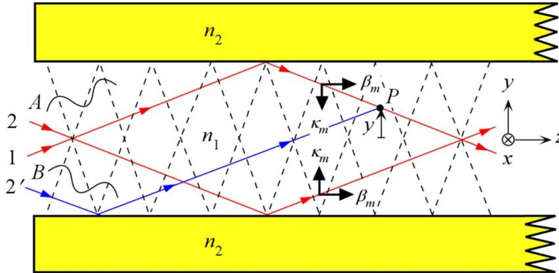
We can identify upward (A) and downward (B) traveling waves in the guide which interfere to set up a standing wave along  $y$  and a wave that is propagating along  $z$ . Rays 2 and 2' belong to the same wave front but 2' becomes reflected before 2. The interference of 1 and 2' determines the field at a height  $y$  from the guide center. The field  $E(y, z, t)$  at  $P$  can be written as
