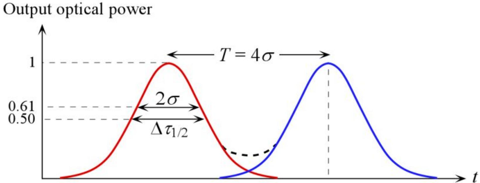
A Gaussian output light pulse and some tolerable intersymbol interference between two consecutive output light pulses (y-axis in relative units). At time  $t = \sigma$  from the pulse center, the relative magnitude is  $e^{-1/2} = 0.607$  and full width root mean square (rms) spread is  $\Delta\tau_{\text{rms}} = 2\sigma$ . (The RTZ case)
