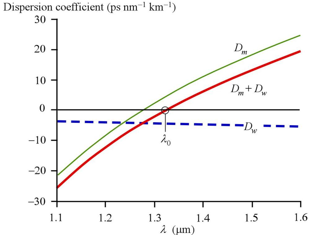
Material dispersion coefficient ( $D_m$ ) for the core material (taken as  $\text{SiO}_2$ ), waveguide dispersion coefficient ( $D_w$ ) ( $a = 4.2 \mu\text{m}$ ) and the total or chromatic dispersion coefficient  $D_{ch}$  ( $= D_m + D_w$ ) as a function of free space wavelength,  $\lambda$
