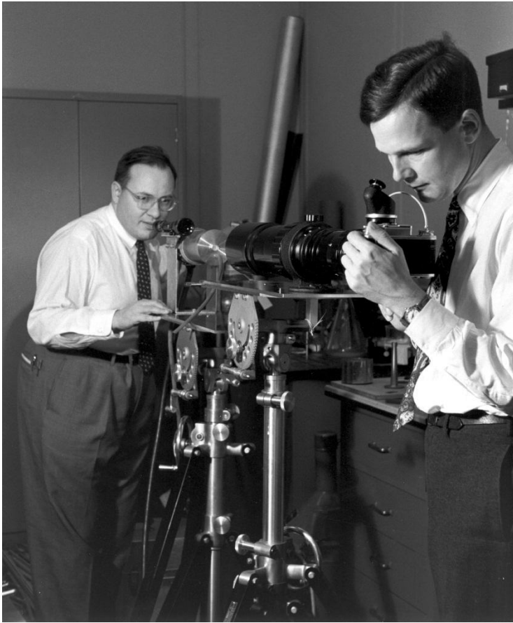
Arthur L. Schawlow is adjusting a ruby optical maser during an experiment at Bell Labs, while C.G.B. Garrett prepares to photograph the maser flash. In 1981, Arthur Schawlow shared the Nobel Prize in Physics for his "contribution to the development of laser spectroscopy" (Courtesy of Bell Labs, Alcatel-Lucent)
