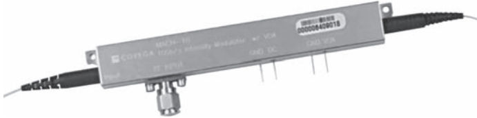
Twenty GHz analog Mach–Zehnder intensity modulator for use at 1550 nm, with half-wave voltage of 3.5 V. The modulator uses titanium-diffused Z-cut LiNbO 3 . (Courtesy of Thorlabs.)
