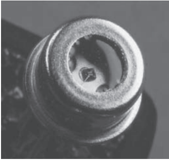
This VCSEL diode provides a single transverse mode emission 795 nm. The spectral width is less than 100 MHz, and the output power is 0.15 mW at 2 mA. (Courtesy of Vixar Inc.)
