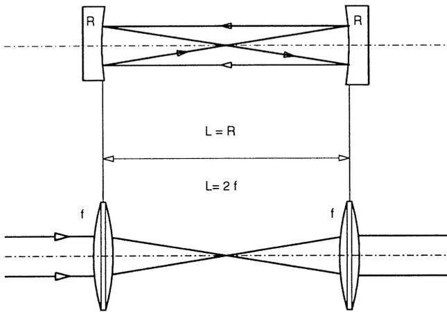
Fig. 24: Spherical resonator with equivalent lens guide.
