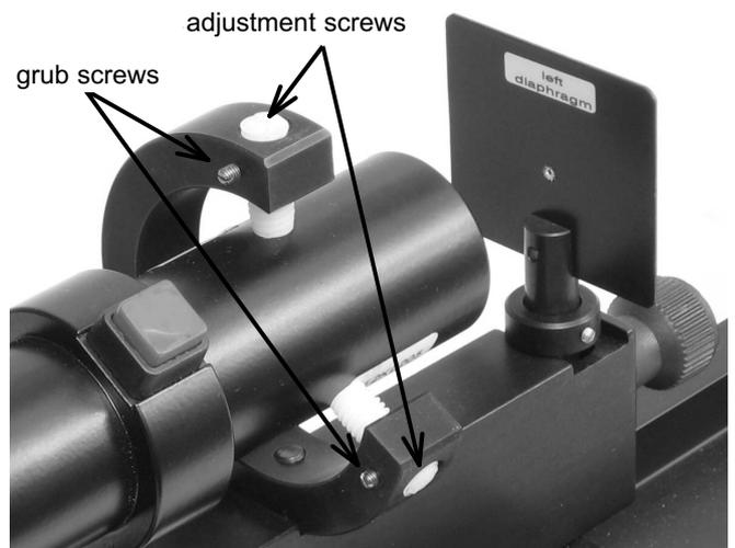
Fig. 4: Adjustment screws.
