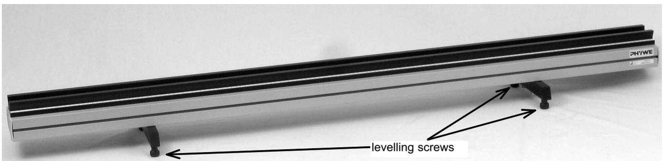
Fig. 2: Levelling screws of the optical bench.
