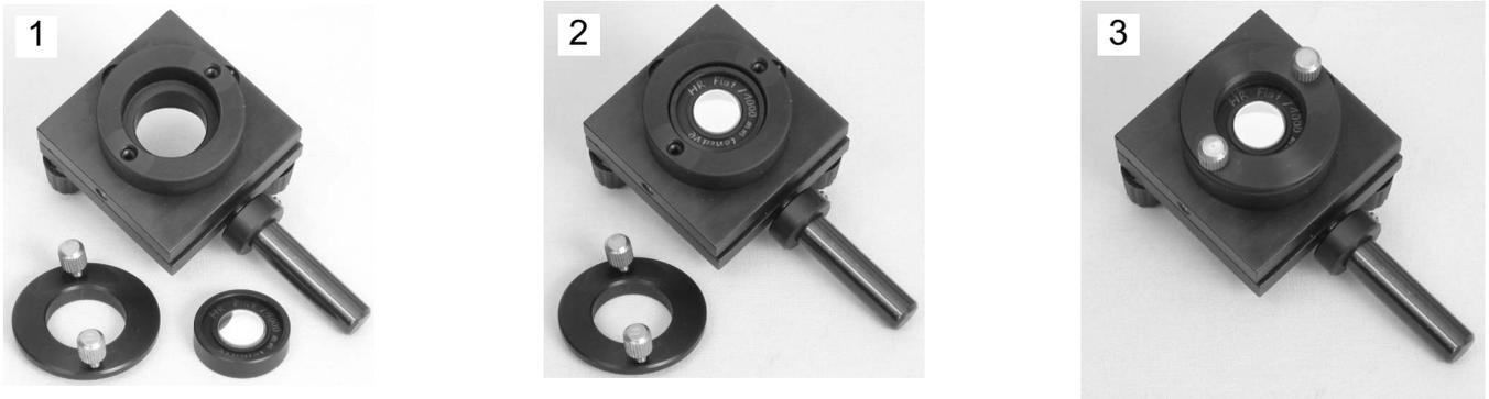
Fig. 9: Assembling the resonator mirror.
