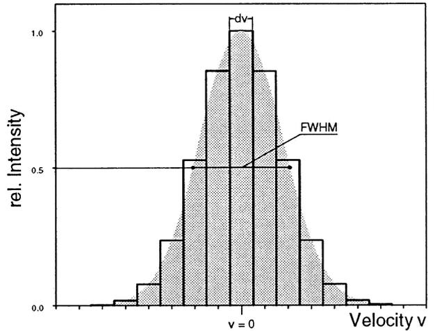
Fig. 20: Inhomogeneous line profile, speed intervals  $dv$ .
