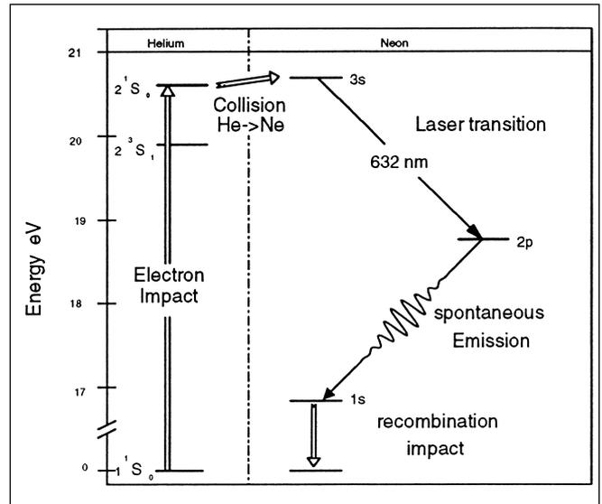
Fig.16: Excitation and laser process for the visible laser emission
