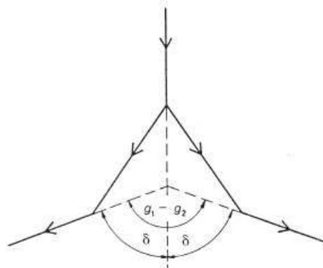
Fig. 6: Measurement of the angle of minimum deviation.
