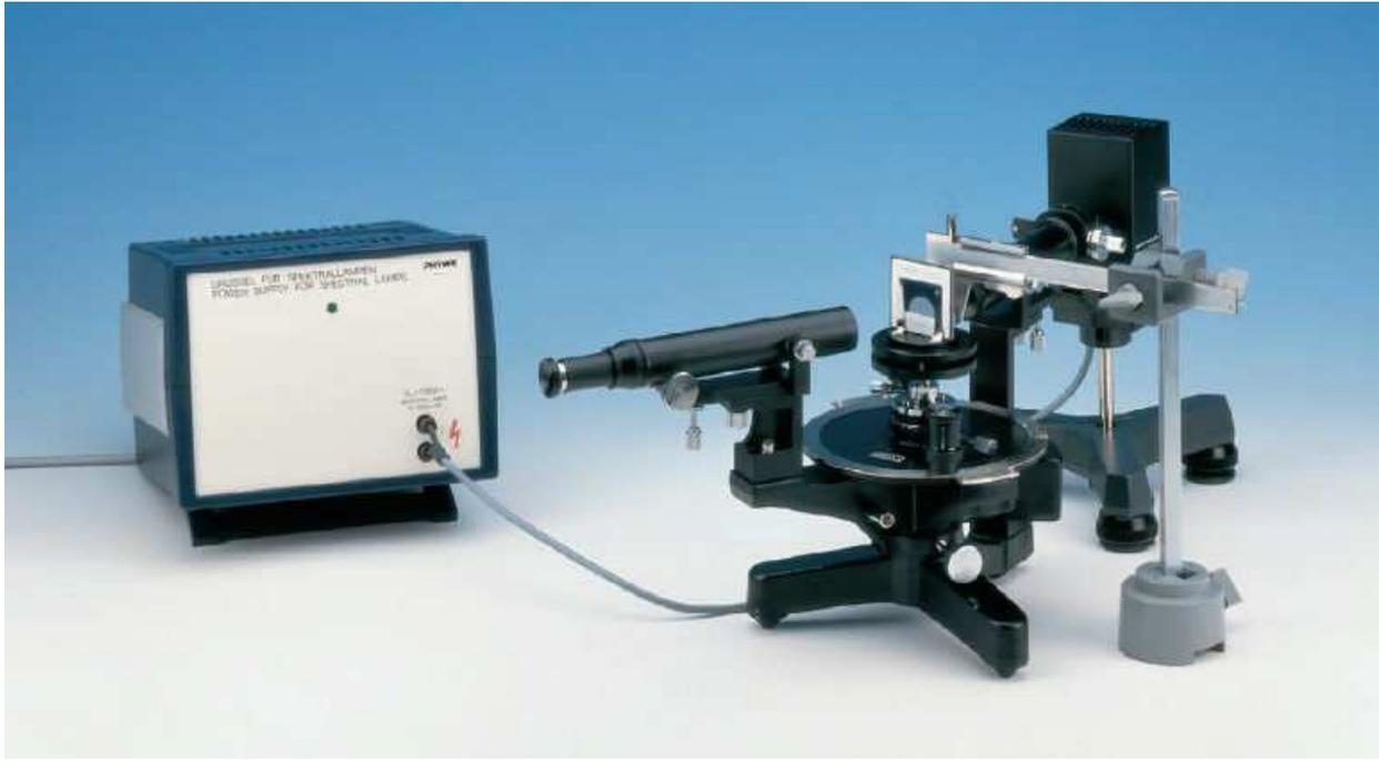
Fig. 3: Experimental set-up with vernier used auxiliary slit to determine the resolving power.
