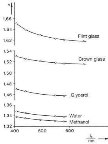
Fig. 4: Dispersion curves of various substances.
