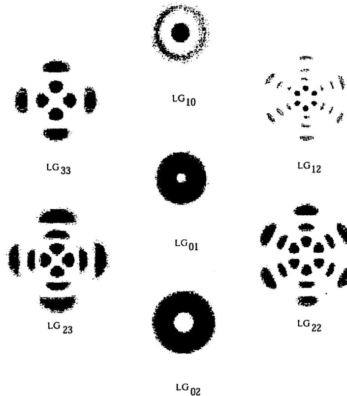
Fig. 8: Intensity distribution of the Laguerre-Gaussian resonator modes.
