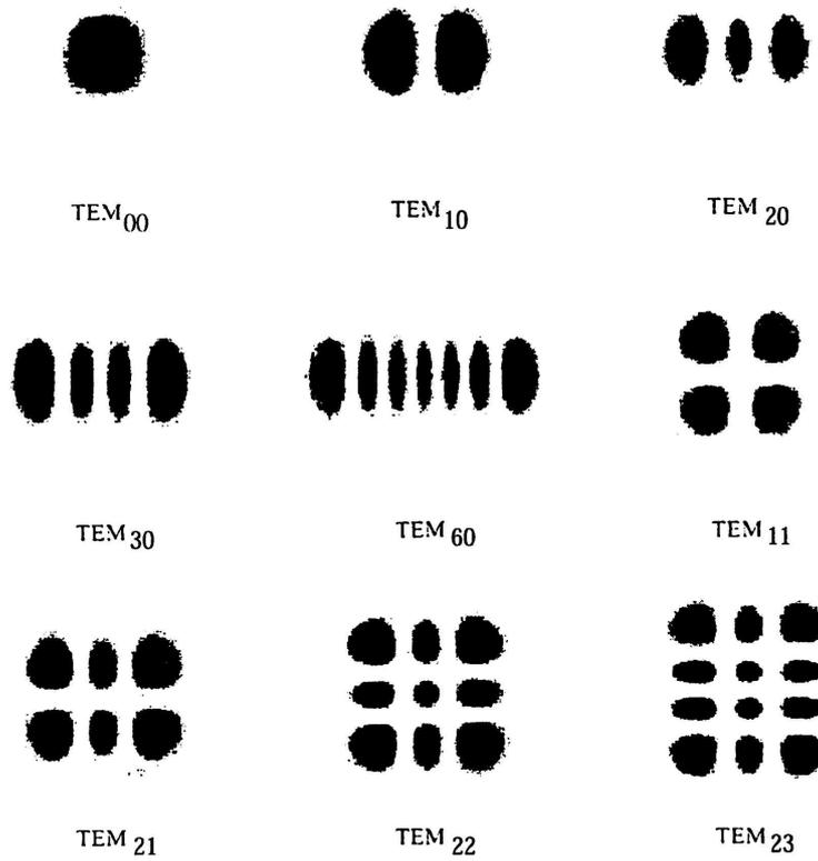
Fig. 7: Intensity distribution of the Hermitian-Gaussian resonator modes.
