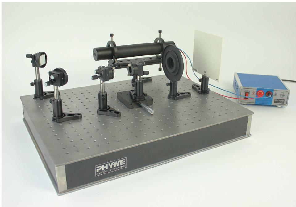
Fig. 1a: Experimental set-up of a Fabry-Perot interferometer for the investigation of the mode spectrum of an optical resonator.
