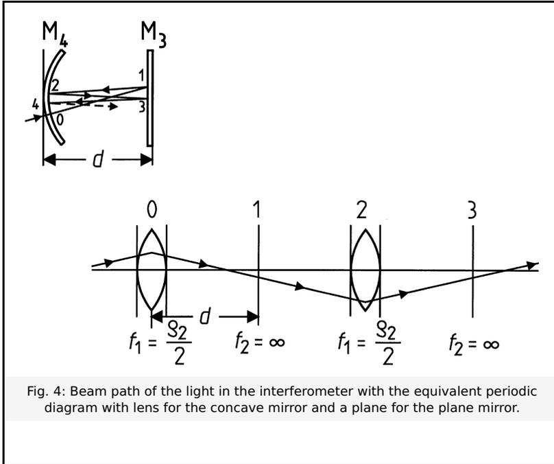
Fig. 4: Beam path of the light in the interferometer with the equivalent periodic diagram with lens for the concave mirror and a plane for the plane mirror.
