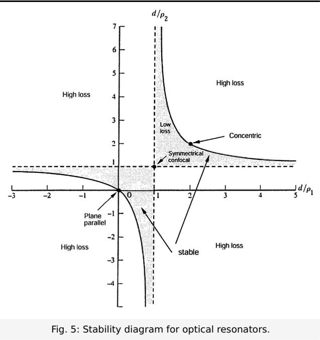
Fig. 5: Stability diagram for optical resonators.
