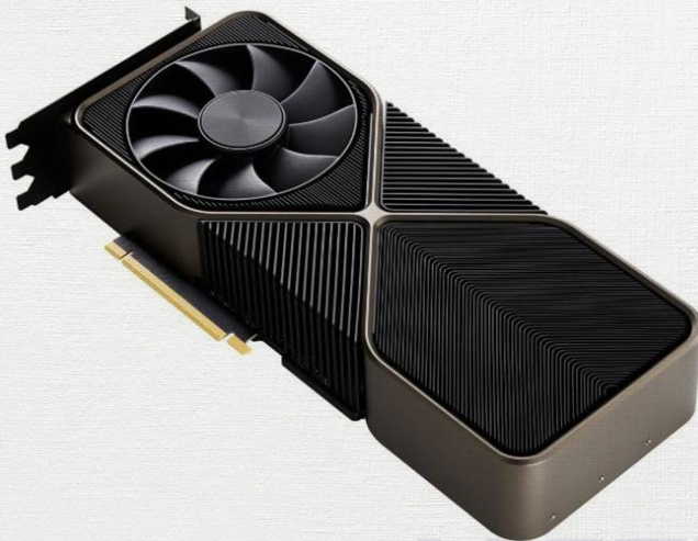
Figure 7: GeForce RTX 3090: 10496:328:112:328:82 shader processor:texture mapping:render output:tensor cores:raytracing cores @1395MHz (1695MHz boosted), 24GB RAM@19500MT/s. 35580 GFLOPS, 285480 Tensor GFLOPS
