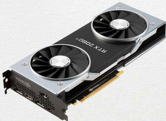
Figure 6: GeForce RTX 2080 Ti: 4352:272:88:544:68 shader processor:texture mapping:render output:tensor cores:raytracing cores @1350MHz (1545MHz boosted), 11GB RAM@14000MT/s. 11750 GFLOPS, 94003 Tensor GFLOPS
